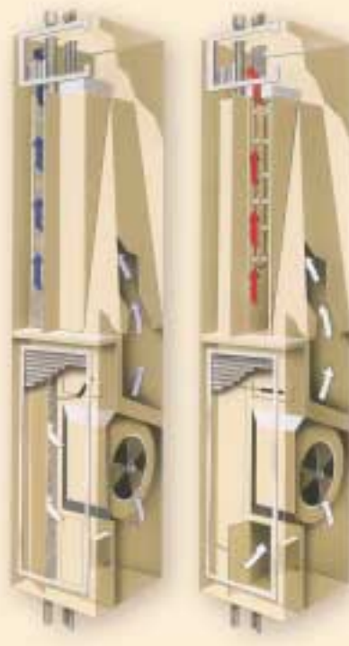
Two-Pipe unit with Electric Heat
