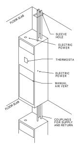
Cut measured riser pipes and the condensate drain line. It is not necessary to have piping inserted the full length of any swaged connection. Deburr and clean the ends of all piping. If the project requires riser extensions due to the floor-to-floor height, this is the time that they should be measured, cut and added to the unit risers. Modifications requiring the extension or shortening of risers are the responsibility of the installing contractor.
