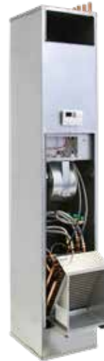
Coil Pack shown halfway in/out of cabinet. The flex hoses facilitate easy slide in/slide-out functionality.
