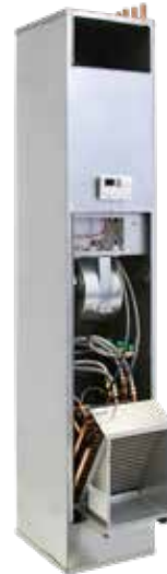
Chassis shown halfway in/out of cabinet. The flex hoses facilitate easy slide in/slide-out functionality.
