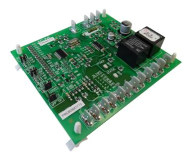
possible damage to the compressor. The threshold temperature is field selectable for 0°, 10°, 20°, 36°, or 125°F. If the sensor drops below (or above 125°) the set temperature twice within 1 hour, the control board will initiate a hard lockout and the alarm contact will energize.
