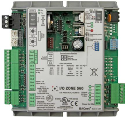
MS/TP, Johnson Controls N2, and Modbus. The protocol of choice for the particular system is selected by simply configuring DIP switches on the DDC control. This flexibility allows one controller to be used in a multitude of buildings which use any of these three common protocols. The control serves as a node of information processing between the Whalen heat pump and the DDC network.
