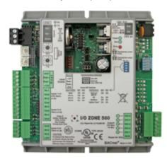
ler is designed to allow the integration of Whalen water source heat pump equipment into DDC systems. The I/O Zone 560 DDC controller has the ability to communicate through a choice of three widely used protocols: BACnet MS/
